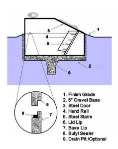
Bolt shelter with straps provided. Slope soil away from shelter.
