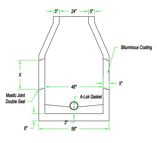
Reinforcement ASTM C-478 Concrete 4000 Minimum PSI Riser Dimension X comes in multiple sizes.
