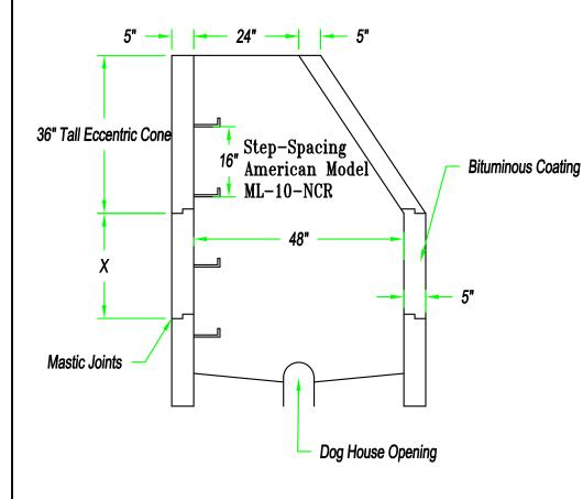
Reinforcement ASTM C-478 Concrete 4000 Minimum PSI Riser Dimension X comes in multiple sizes.
