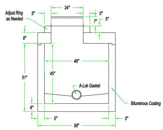
Reinforcement ASTM C-478 Concrete 4000 Minimum PSI
